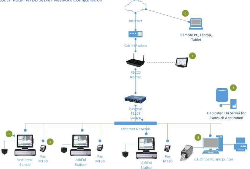
\*All Exatouch bundles, terminals, remote printers, and PC/Laptops running back office must be connected via Ethernet cat 5e/6 cable to the FS108 switch in order to communicate.
